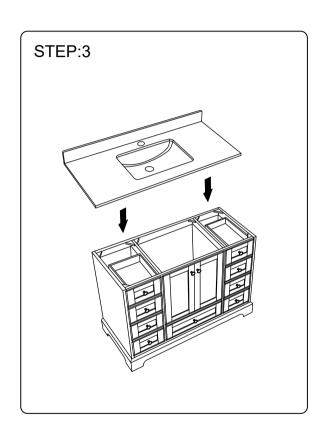
Install countertops with clear or white silicone sealant to seal the top of the cabinets.
