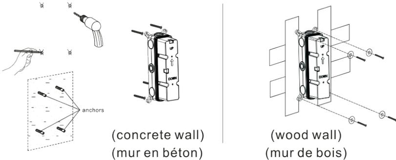
1. Make marks according to the size of the main body valve and then drill anchors into the wall (concrete wall)
