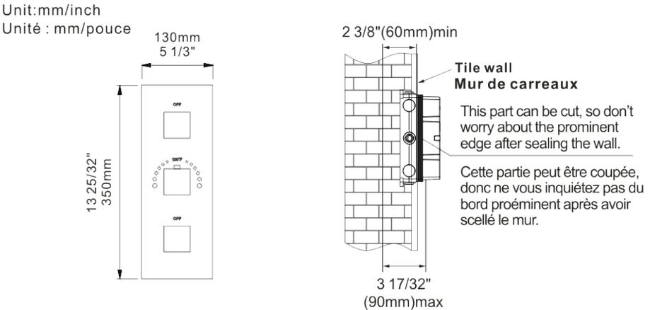
**Notice:** 1. The installation depth of main body should be no less than 2 3/8"(60mm)and no more than 3 17/32"(90mm), including the thickness of tile. Other wise, the deck plate cannot be installed.
