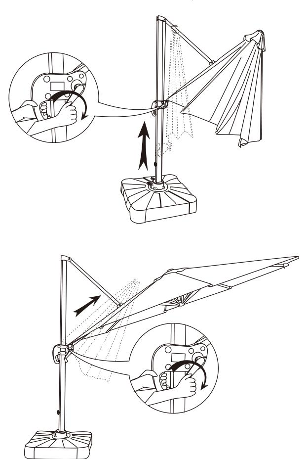
$\textbf{Step 8} \quad \text{The umbrella has 6 position holes on the main pole to lock the canopy at different angles} \; .$
