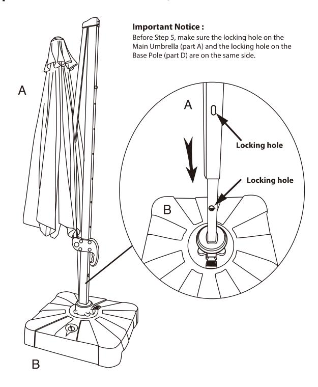
Step 6 Insert the Crank Handle (part J) into the square hole on the Main Umbrella (part A). Screw the Threaded Knob (part I) into the locking hole on the Main Umbrella (part A).
