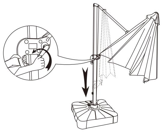
**Step 10** This umbrella has a 360 degree swivel mechanism. Before attempting to turn the umbrella, close the umbrella first and squeeze down the lever with your foot to release the mechanism.
