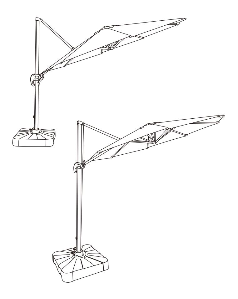
Step 9 Squeezing the trigger before attempting to lower the crank house. Turn the Crank handle counter-clockwise to close the umbrella.
