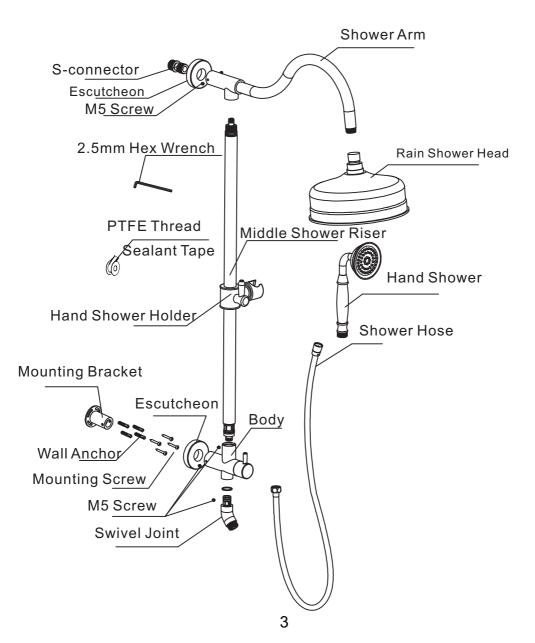
1.As specified in diagram, attach the shower base to the water supply pipes in the wall.
