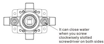
Note: If only close one side that it will cause faucet abnormal outlet water, for normal outlet water please make sure the adjusting position on both sides is open (counterclockwise to open).
