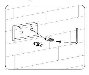
11, Tighten the fitting with an Allen wrench
