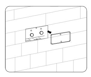
10, The embedded box is installed, waiting for the concrete to solidify Remove the protective cover.
