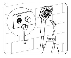
4. Hot water and tap water enter the valve body at the same time and open the shower to discharge water Adjust the temperature, US temperature is set to  $100F^{\circ}$ ; Canada, The European default setting is  $38C^{\circ}$ , the adjustment is complete Install the knob with an Allen key
