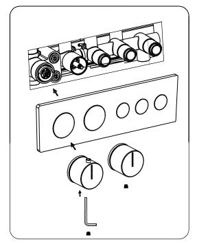
3. Water pipes and valve body pouring concrete, waiting for concrete Curing Follow the instructions in the picture to install the knob.
