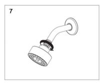
7. Install showerhead use teflon tape on at least the first 3 threads and screw on the shower head using a wrench.
