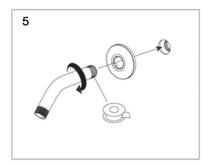
5. Install the shower arm and flange. Slide the flange onto the shower arm and telflon tape at least the first 3 threads of the end going into the wall (pipedope is recommended also for any connections in the wall) tighten arm securely.
