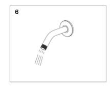
6. Turn on water to flush out any debris that may be in the lines.
