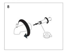
8. Install tub spout use teflon tape on at least the first 3 threads and screw on the tub spout securley.
