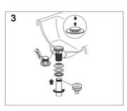
3. Apply a thin bead of putty/silicone onto the flange insert the drain body into the sink slide the nut up and thread it counter clockwise on the drain body underneath the sink until it is firmly screwed to the bottom of the sink Do not over tighten the nut.
