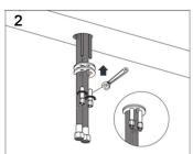
2. Install the rubber washer, metal washer, and mounting nut onto the faucet shank in that order underneath the countertop. Tighten down the nut ensuring the faucet is in the proper position.
