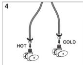
Attach the open ends of the water supply lines to the hot and cold shut-off valves and tighten with a adjustable wrench.
