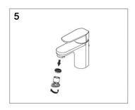
5. Remove the aerator from the spout, turn on the shut off valves. Check for leaks on supply line connections.
