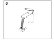
6. Flush out the water lines of any possible debris. Close the pop up assembly and fill the sink with water to check the drain for leaks.
