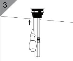
Tighten the two screws on mounting nut (E) with a screwdriver.
