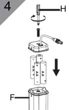
To use the small Screwdriver (H) that applied to open the battery box (F), insert 4pcs of alkaline batteries, make sure that the positive and negative poles must be installed properly. and then lock the battery box.
