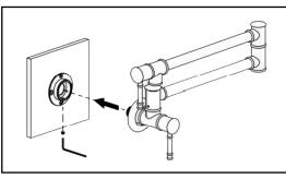
2. Wrap the end of the 1/2" IPS nipple with teflon tape covering at least the first three threads (thread sealant is also recommended for any connections in the wall), screw the faucet body nipple to the mounting base plate, assuring it is in the correct position when faucet body is pulled out straight. Insert the set screw into the bottom of the mounting base plate and tighten. Place the finish trim plate onto the mounting base plate.
