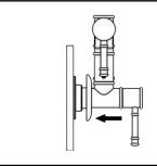
3. Remove aerator from faucet, turn water on to flush any possible debris in the cold water line and check for any leaks at the connections. Place the finish trim plate onto the mounting base plate.
