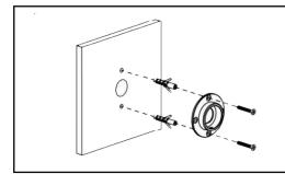
1. Place the mounting plate against the wall and mark out the holes. Using a 6mm drill bit, drill out the holes and insert the plastic anchors (a hammer may be needed to insert fully into wall). Place the mounting base plate over the plastic anchors and mount to the wall using the anchor screws.
