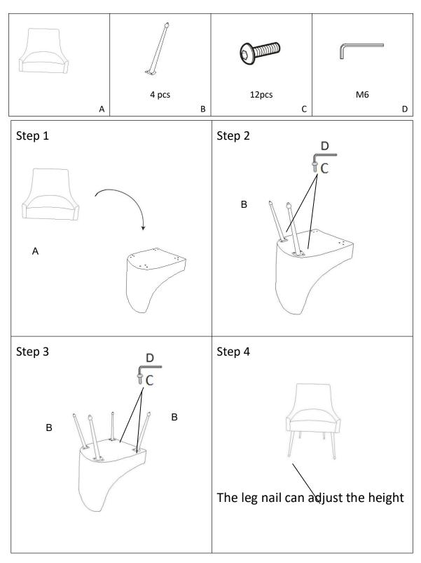
Note: Put all the screws into the hole site, And then tighten them. Do not tighten one by one
