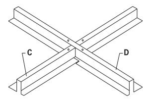
**Step 1:** Place Lower Cross Leg (C) on the ground, line up notches and place Upper Cross Leg (D) over the Lower Cross Leg (C)
