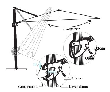
**Step 2:** To open the umbrella, squeeze the Glide Handle and grip together and slide up or down the pole to achieve the desired tilting angle. Release the grip to lock into place. To open the canopy, turn the crank handle clockwise until the canopy is fully open.
