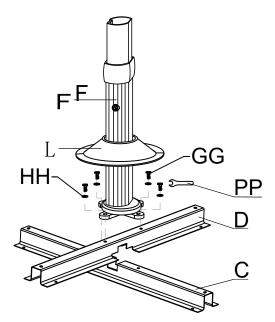
**Step 2:** Attach the Holder Pole (F) to the base by using the Bolts (GG) and Washers (HH), hand tighten only. Adjust the Holder Pole (F) to be sure it is positioned correctly on the base and finally tighten all bolts. Be careful not to over tighten.
