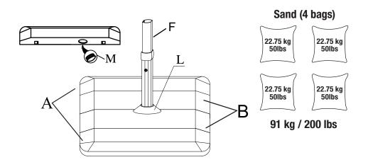
**Step 3:** Place Blow Molded Base (A & B) on the cross bar assembly and fill with sand and water, cover with caps (M). Place Pole Support Cup (L) onto Holder Pole (F) and lay on top of Blow Molded Base (B).
