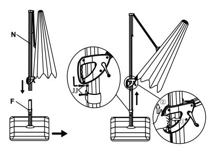
**Step 4:** Insert Umbrella Frame with Canopy (N) into the Holder Pole (F). Slide the holder pole collar onto the holder pole at the same time. Tighten the two Hex Bolts (JJ) into the holder pole to secure the umbrella.
