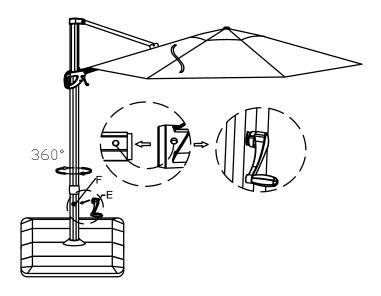
**Step 4:** To rotate umbrella, insert the crank handle (E) into holder pole (F) and turn to desired position.
