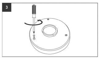
Place the solar panel face-down on a soft, clean surface. Remove (3) screws from the bottom of the panel.
