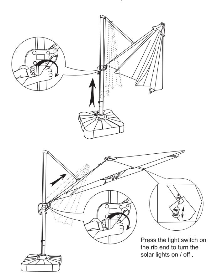
$\textbf{Step 11} \hspace{0.1in} \textbf{The umbrella has 6 position holes on the main pole to lock the canopy at different angles} \hspace{0.1in}.$
