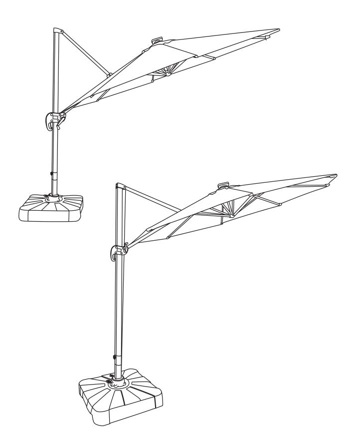
Step 12 Squeeze the trigger before attempting to lower the crank house. Turn the Crank handle counter-clockwise to close the umbrella.
