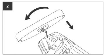
Align the notches on the solar panel with the grooves on the top of the umbrella, hide the plug and wires inside the hollow space. Turn the solar panel clockwise to lock into place; do not over-tighten.
