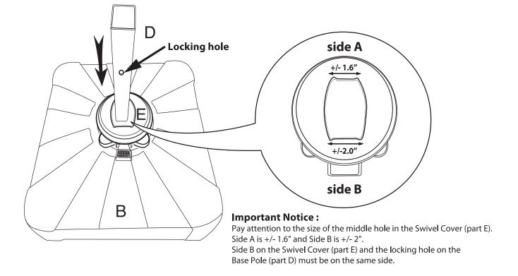
**Step 5** Place the lower pole (part M) on the base as below.
