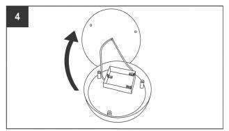
Carefully lift the bottom of the panel, ensuring the wires remain intact. Gently remove the old batteries. Paying attention to the positive and negative terminals, insert new batteries.
