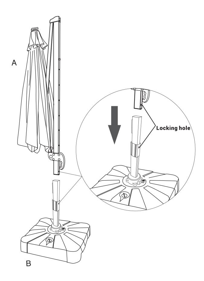
Step 9 Insert the Crank Handle (part J) into the square hole on the Main Umbrella (part A). Screw the Threaded Knob (part I) into the locking hole on the Main Umbrella (part A).
