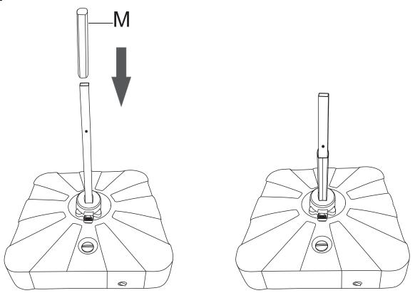
Step 6 Fix the plastic connector (part L) on the top of the lower pole (part M). Make sure the two holes are on the same side as below.
