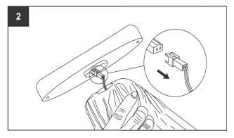
Carefully disconnect the plug from the socket by pressing the tabs surrounding the connection point. Pull apart by holding the plug, never pull on the wires.
