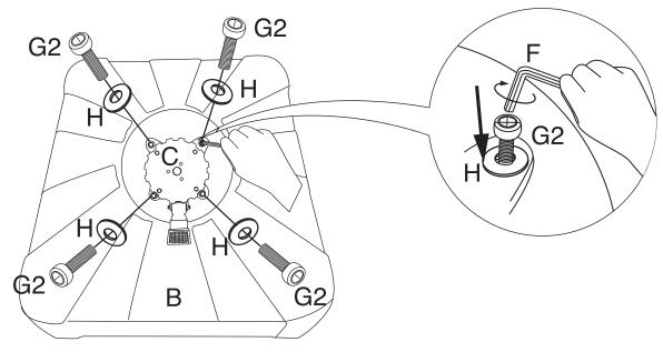
Step 3 Attach the Base Pole (part D) on top of the Swivel Mechanism (part C) with bolts (part G2), washers (part H), and Allen wrench (part F).
