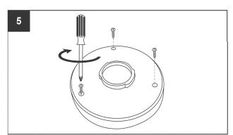
Carefully replace the bottom of the panel and align the screw holes. Secure the panel with the screws removed in step 3. Do not over-tighten the screws.
