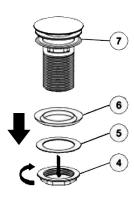
Clockwise rotate and take off nut and gaskets as picture show
