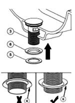
Put the gaskets 6 and 5 onto the thread of the pop up part as the arrows show
