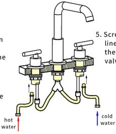
5. Screw the water supply lines to the faucet body, the handles and the stop valves
