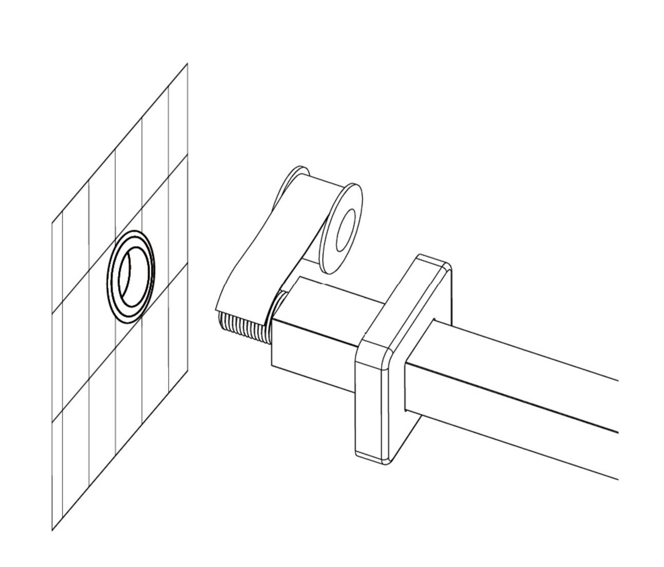
2. Wrap teflon tape on threaded connector
