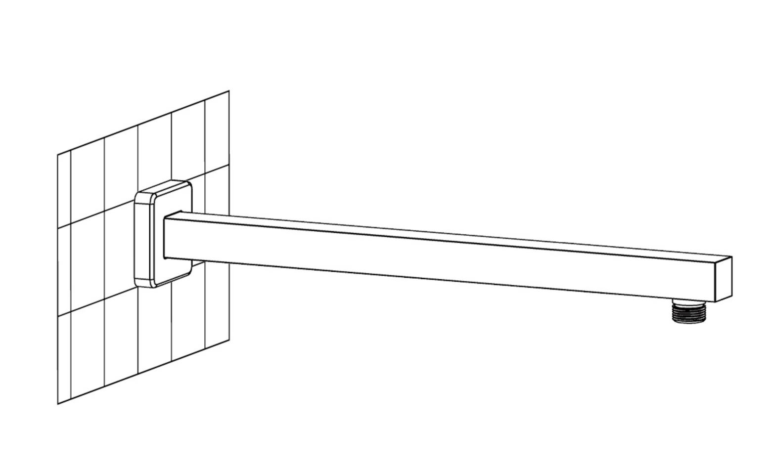
3. Install shower arm and move flange to cover the hole on wall
