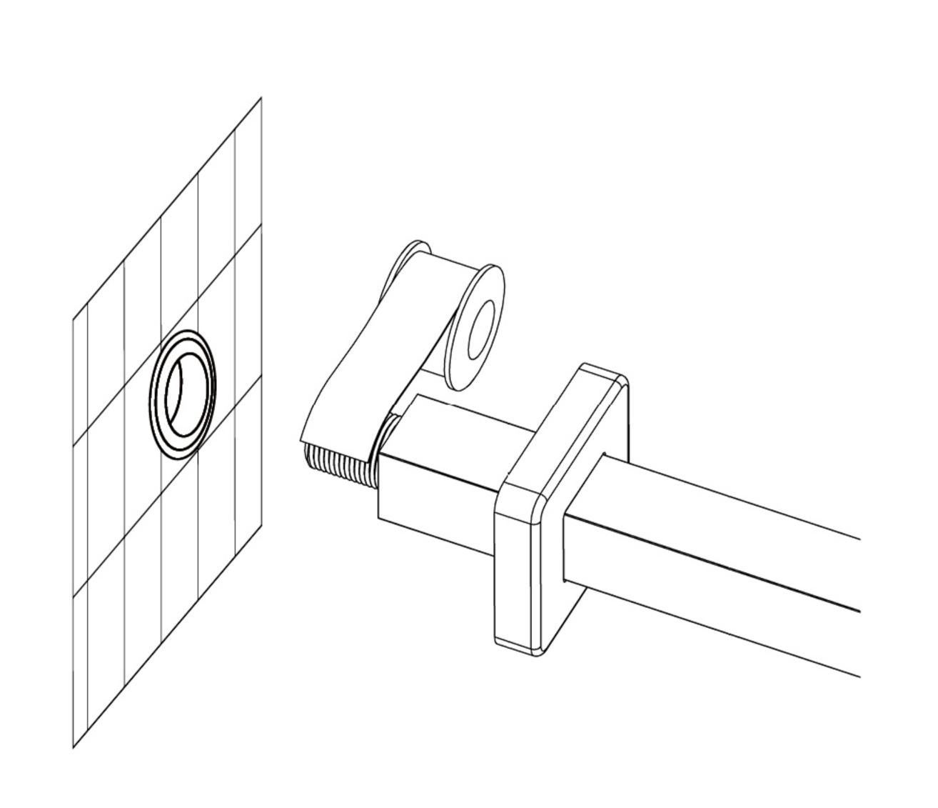
2. Wrap teflon tape on threaded connector
