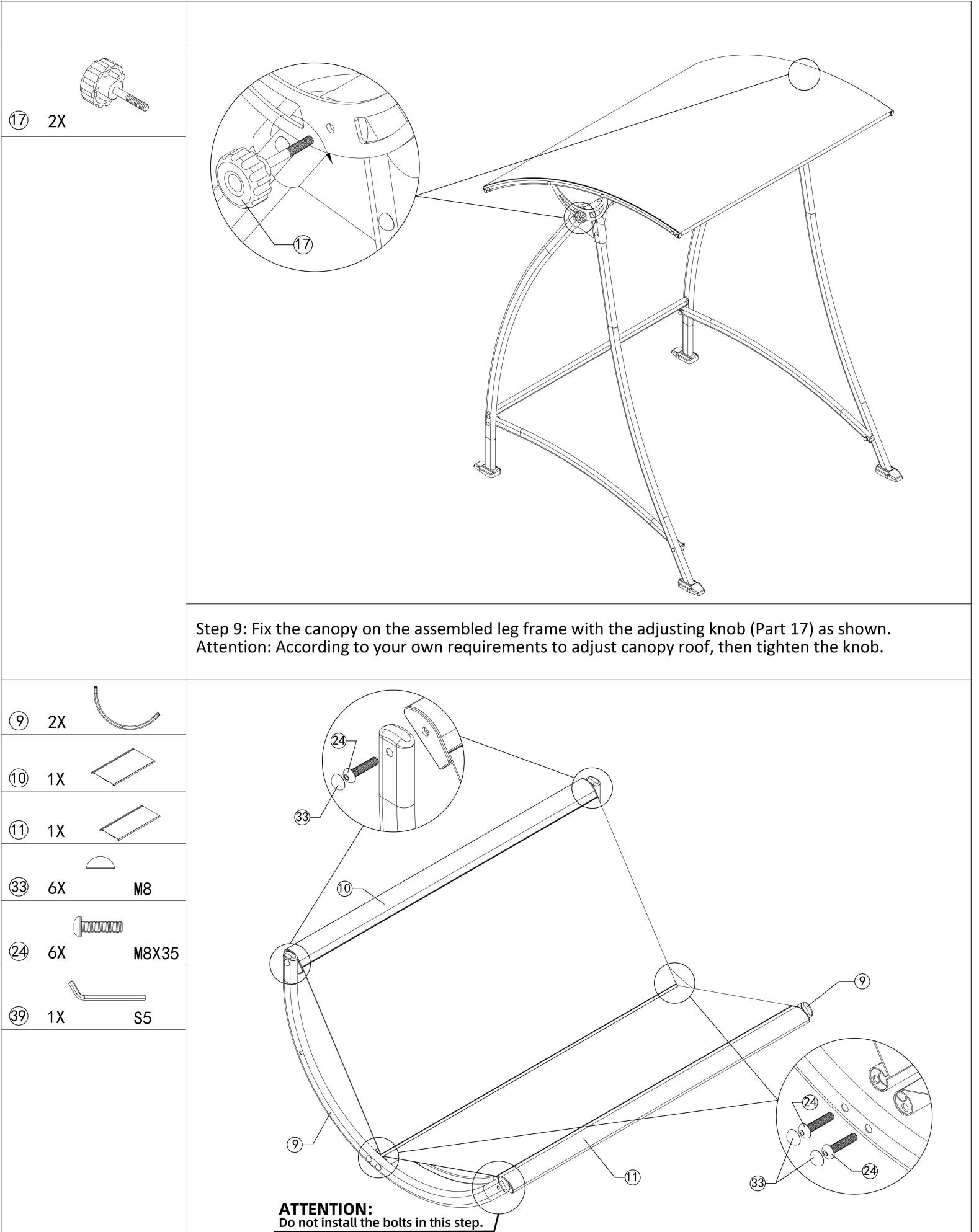
Step 10: Use bolt #24 to secure fixing tube (Part 9) on back (part 10) and seat (Part 11) as shown, secure with bolts and nuts as required (After all the bolts are assembled in place, tighten them together, finally cover the caps).
