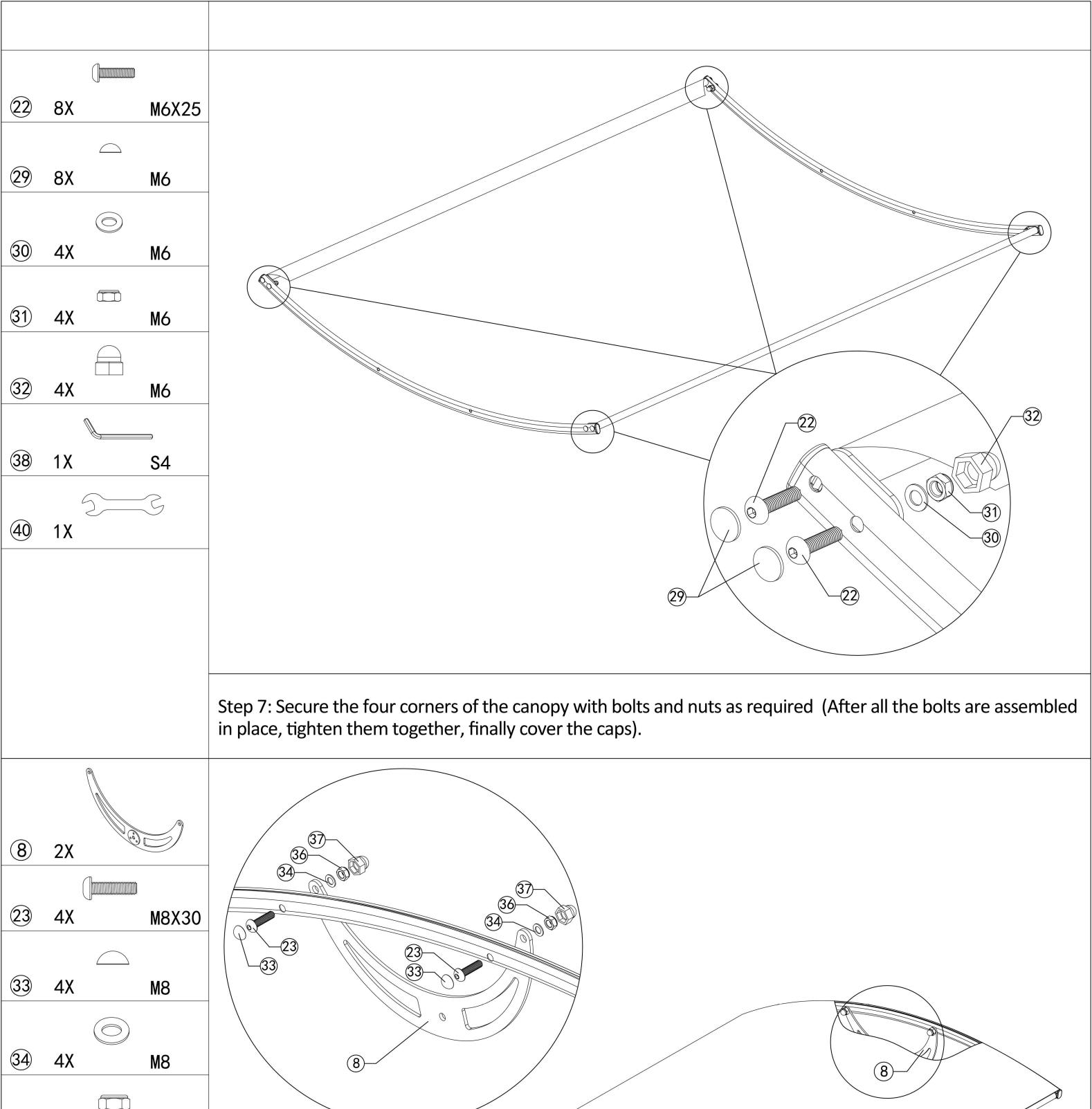
Step 8: Install Part 8 to top canopy. Align the holes and secure with bolts and nuts as required as required (After all the bolts are assembled in place, tighten them together, finally cover the caps).
