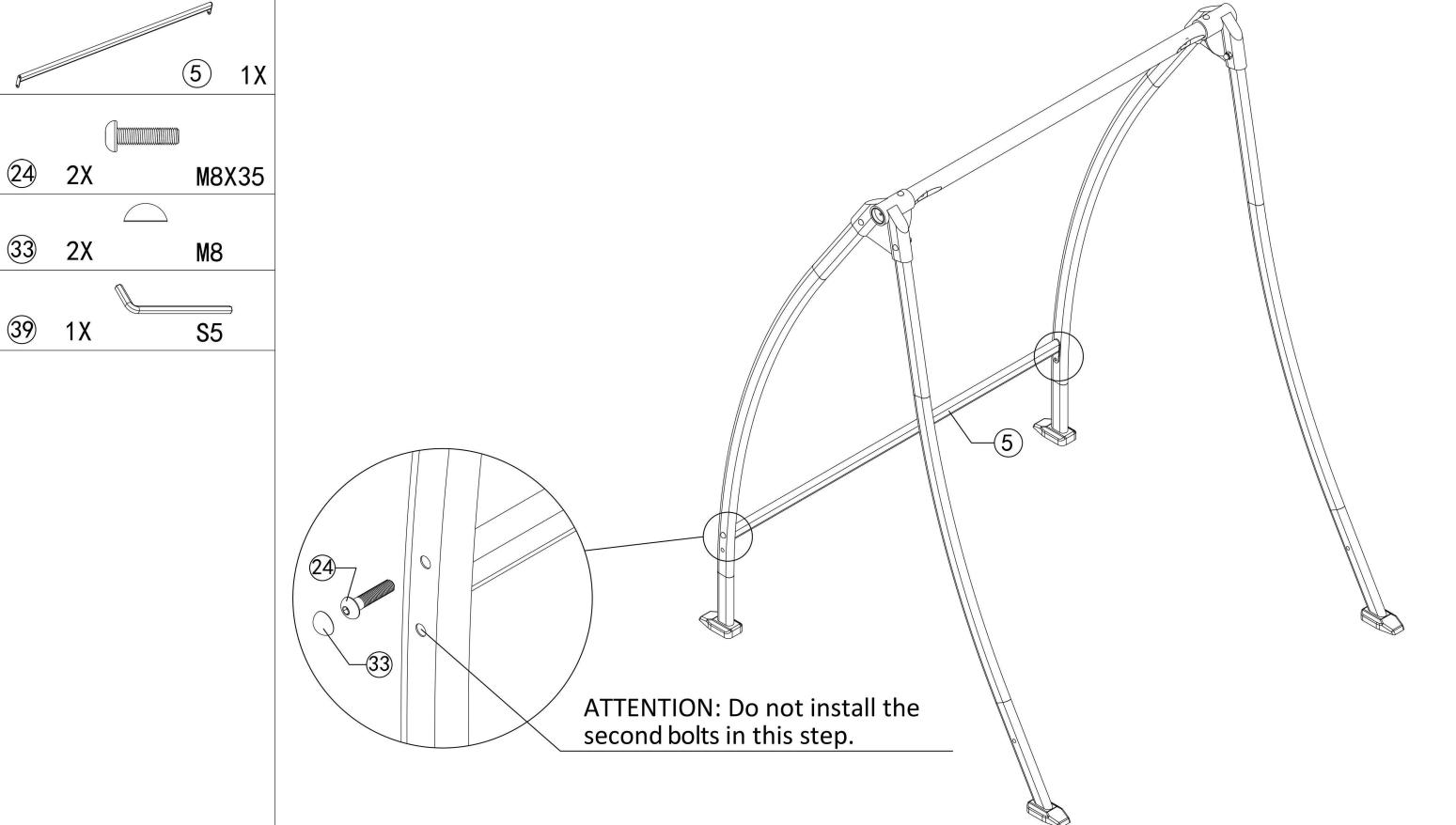
Step 4: Connect the bar (part 5) to the rear leg tubes (Align the first holes and fix the bolts) as shown. After all the bolts are assembled in place, tighten them together, finally cover the caps.
