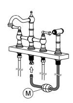
Conect the Spray Hose to quick connector (C). Then install the Weight (M) to the proper place on the Spray Hose. Product install is complete
