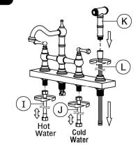
Connect the faucet with hot and cold water supply valve by using hose(I&J), connect the Sprayer (K) to the Spray Hose (L) then put it into the Sprayer Base and ready for the next step.
