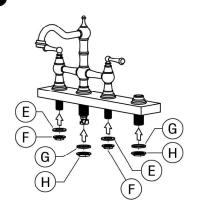
Tighten the faucet and the sprayer base by using small Nut (F) and a large Nut (H), Rubber Washer (G) are required between the Nuts and the fixing plate.
