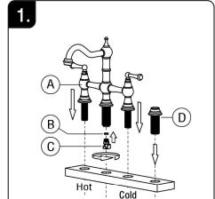
Connect the Quick Connector(C) to the Faucet (A) and sealed it with a Small Washer (B), then put the faucet and the Sprayer Base(D) into the mounting hole, after that, ready for the next step.
