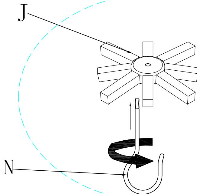
Connecting the Hook N to the Top Connector J.
