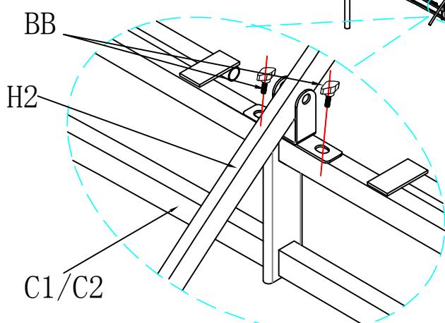
Assemble this part into the Beam(C1/C2) with the end of H2 by using screws BB.
