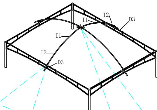
And assemble it to Beam D3 and the middle curtain bar E2 with the side of I2 by using screws BB.
