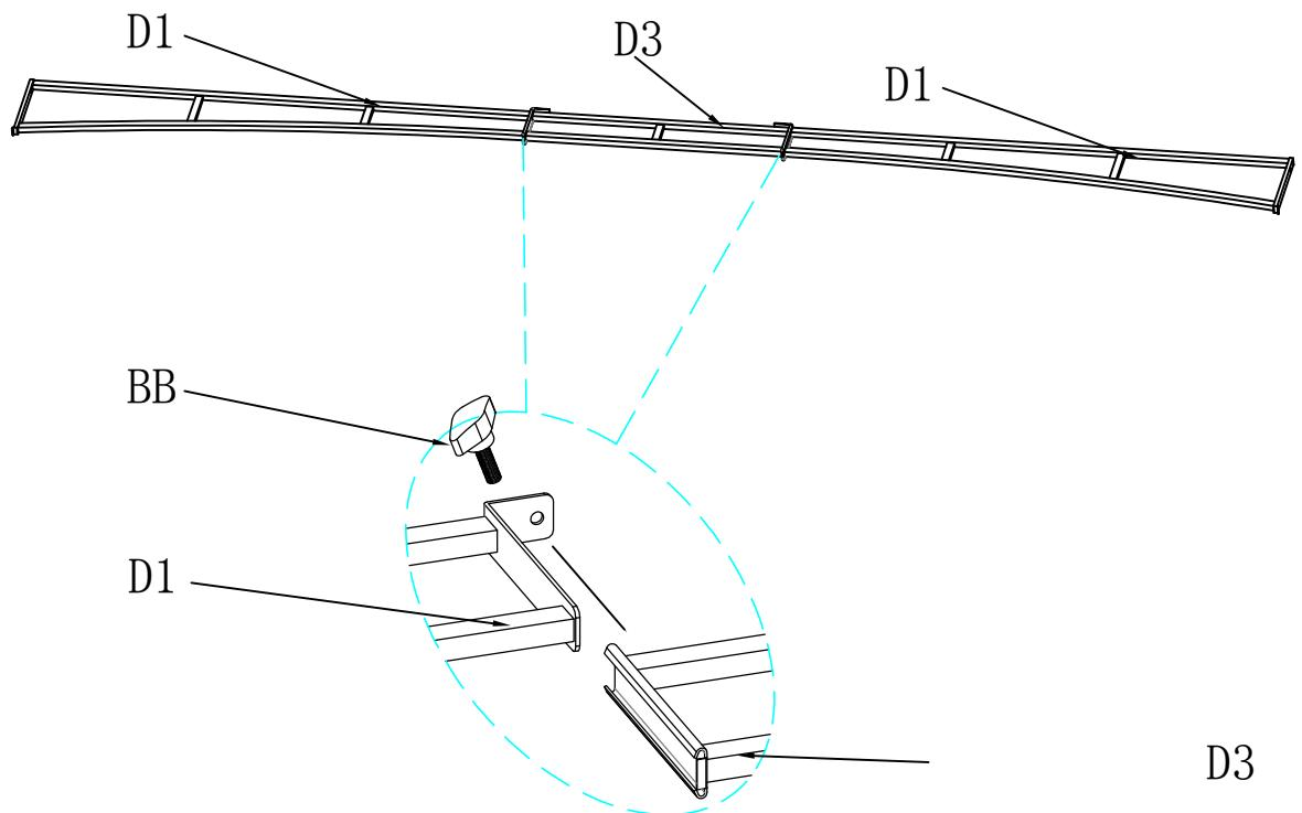
Please find 2 PCS of D1 and assemble them into each end of D3 by using screws BB.
