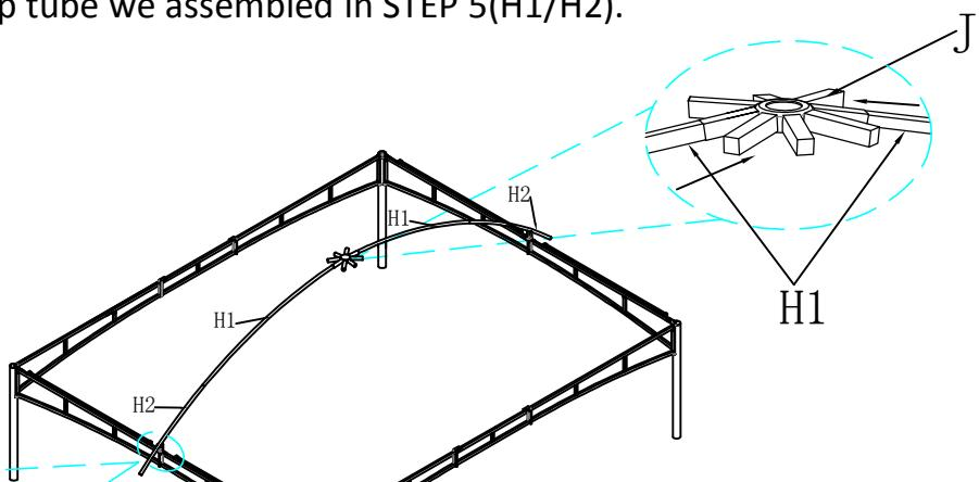
And assemble this part into the Top Connector J with the end of H1.
