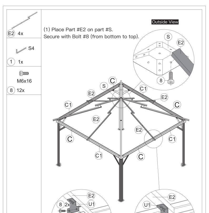
(2) Connect Part #E2 and the Assembled Beam(C&C1) with part #U1. Secure with 2 Bolts #8.
