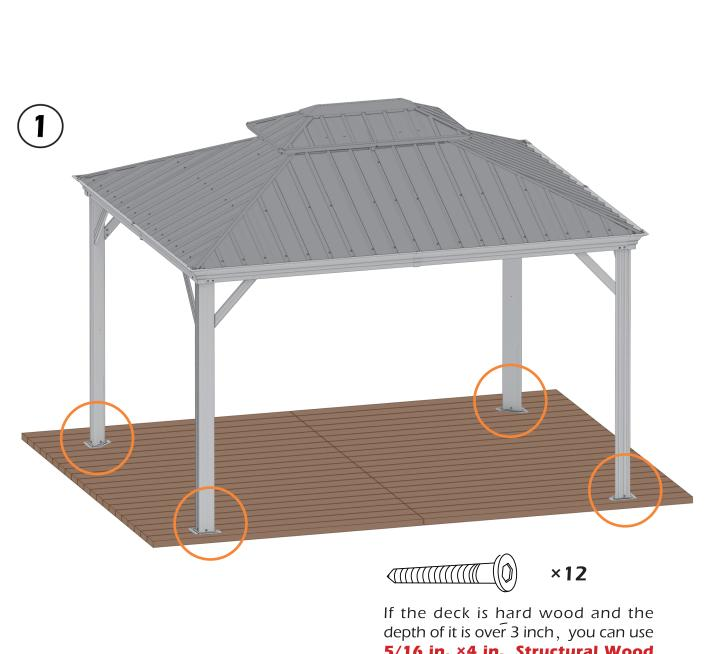
depth of it is over 3 inch, you can use 5/16 in. ×4 in. Structural Wood Screw to mount the gazebo.
