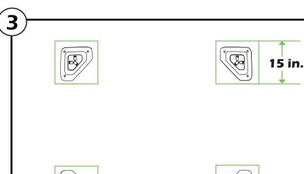
Or you can make a concrete footing for gazebo,  $15 \times 15 \times 15$  inches is recommended use expansion bolts to mount the pergola like (2) shows.
