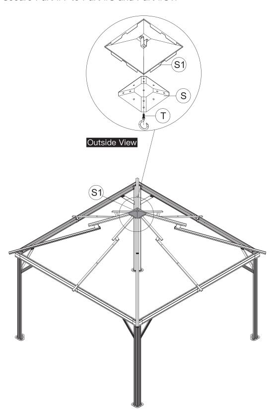
ATTENTION: The holes of Part #S and Part #S1 need to be aligned, on the same vertical line.
