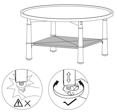
Adjust the table so that it is leveled, then fully tighten all the bolts
