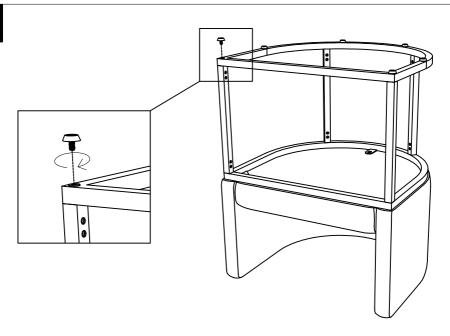
When needed, adjust the height of feet glides to help level the chair.
