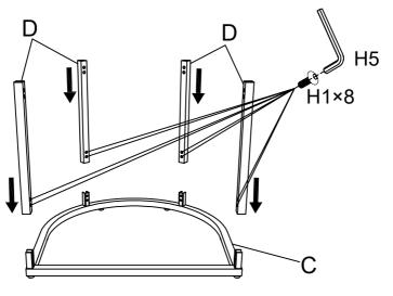
Tighten the bolts to 80% tightness.
