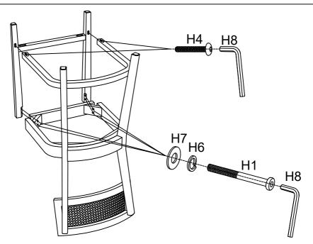
Tighten the bolts to 80% tightness.
