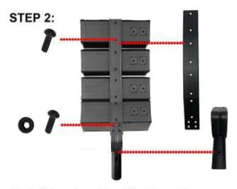
Attach the long bracket and short bracket to the array speaker, secured with screws and nuts.
