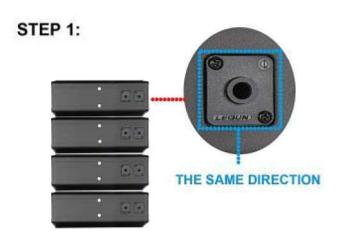
Align four identical speaker. The icon of each should be placed at the same direction with words "LEQUN" on the left bottom.
