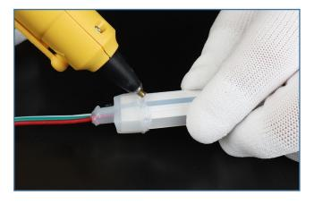
**Step 6 -** Install end caps with silicone glue on both sides.
