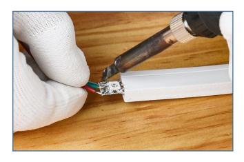
**Step 3 -** Melt the solder joint of the LED strip and remove the wire.
