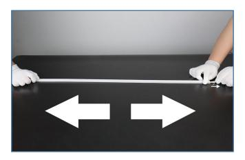
**Step 2 -** Two people straighten the channel and pull the LED strip into it.
