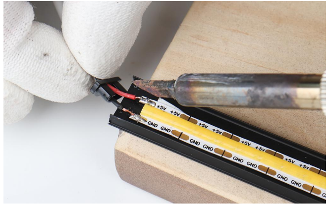
Step8 - Connect the wire to the LED strip.
