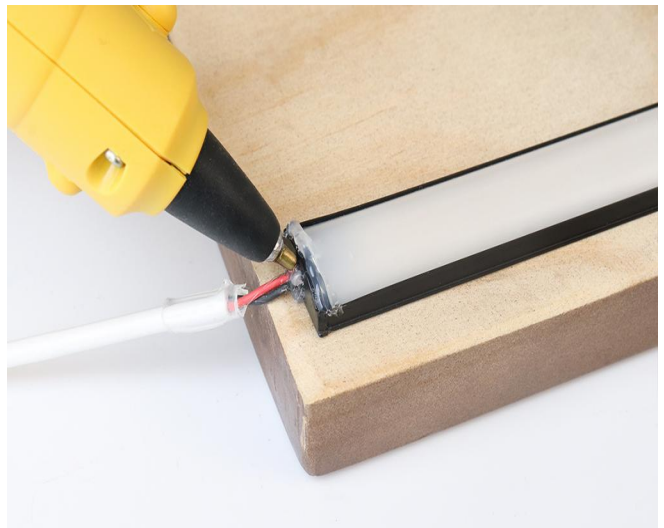
Step10 - Install end caps on both sides (The gap can be sealed with hot melt glue).
