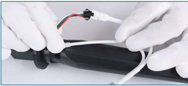
Step 11 - Connect the controller.
