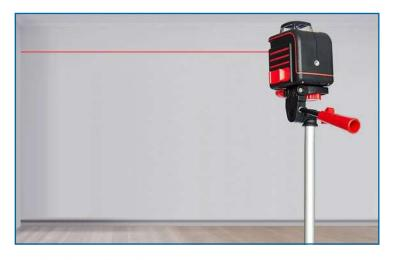
Step 1 - Use a laser level to Step 2 - Snap a chalk line. outline the position of the L tee.
