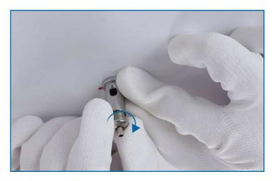
**Step 6 -** Screw the cover onto the tensioner.
