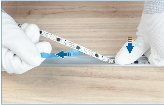
Step 3 - Attach the strip to the LED channel.
