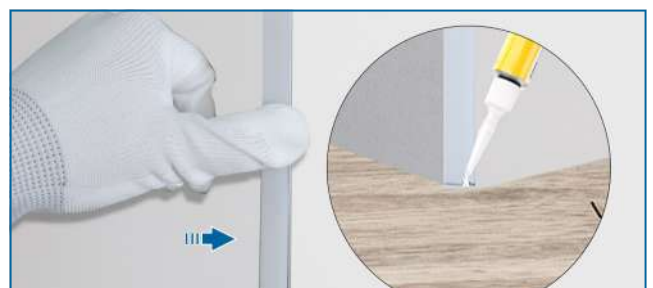
Step 10 - Apply silicone sealant to end caps, then press the cover.
