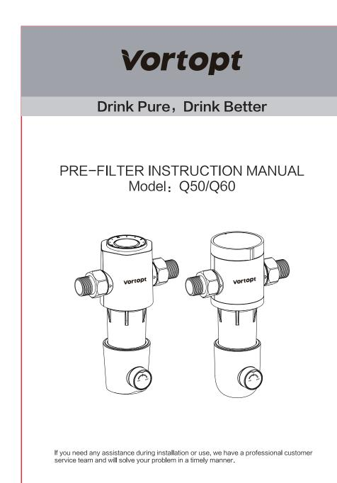
I. Product Introduction The Pre-Filter is mainly used to intercept particle impurities, sediment, rust, floating materials and other pollutants in the water. For downstream plumbing, water purifiers, water heaters, wall-hung furnaces, washing machines, shower baths and other end water-related equipment play a positive protective role.
