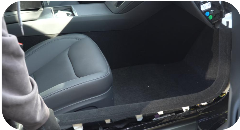
9. Pull down the passenger's side door size
