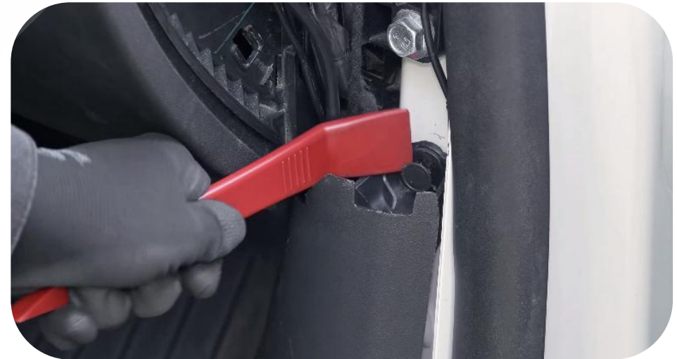
8. Pry open the fixing fastener of the side pedal trim plate, remove the side pedal trim plate and take it out
