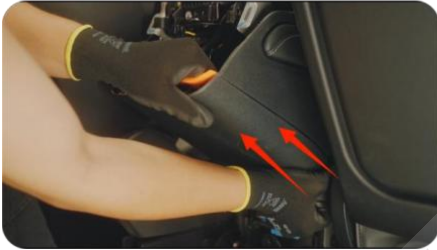
5. Remove the middle trim plate of the air conditioning outlet
