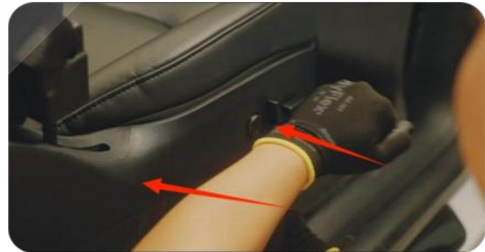
16. Align it with the seat and press it back
