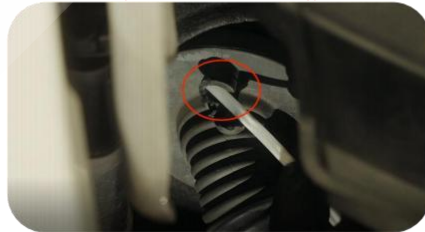
9. Thread the threading tape from the cut position ( Don't break the rubber plug , otherwise it will be difficult to snap it back in)
