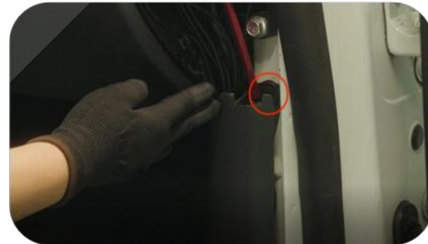
4. Take out the clips on the passenger door trim panel and remove the door sill trim panel.
