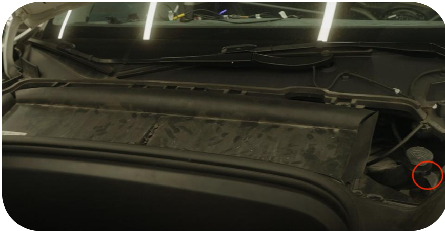
3. Remove the clip on the front trunk
