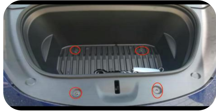
2. Use a No. 10 socket to unscrew the four fixing screws.
