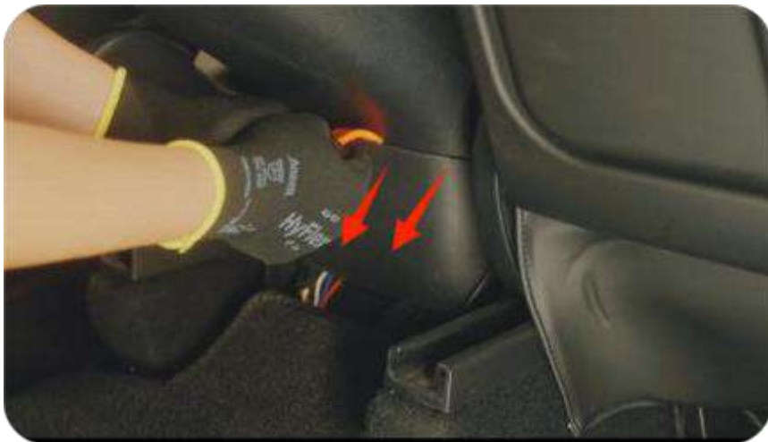
3. Use tools to remove the anti-kick trim panel at the bottom of the saddle.
