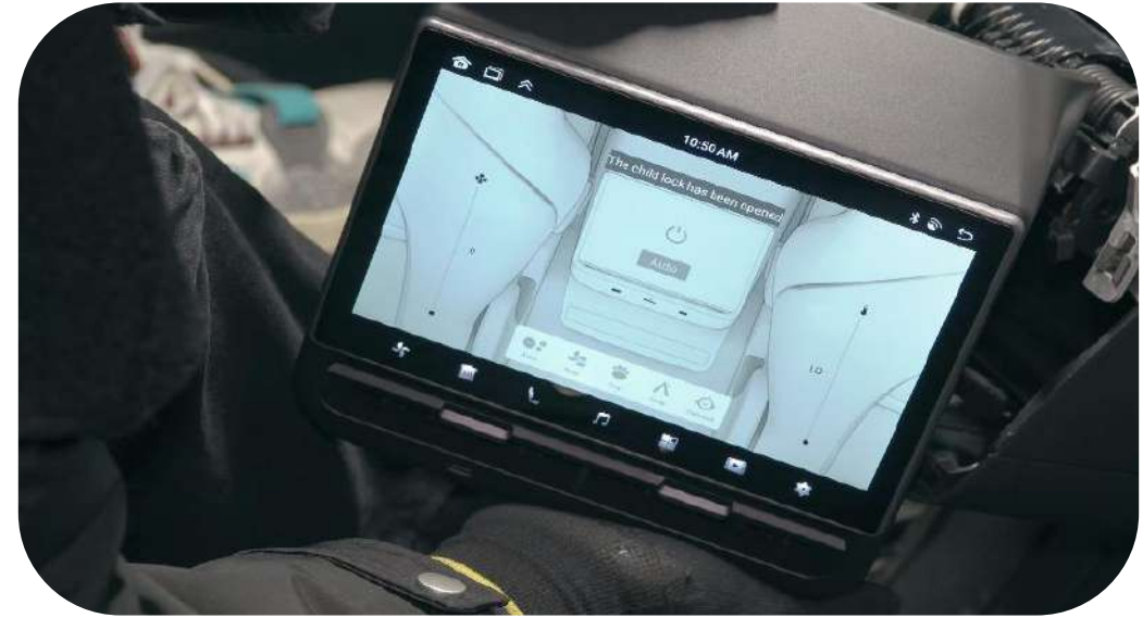
18. Check whether all functions of the screen are normal (See the installation video for details)
