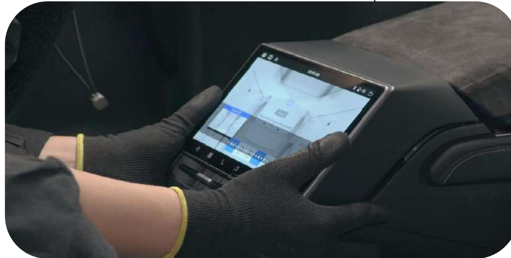
19. Just snap the screen back (During installation, you need to hold the bottom of the screen first and then the top of the buckle. You can watch the installation video to operate)
