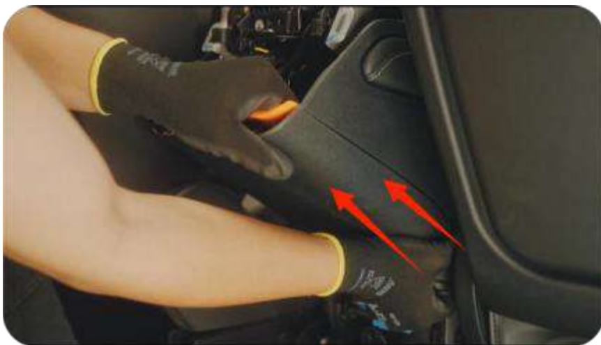
5. Remove the middle trim panel of the rear outlet of the air conditioner.
