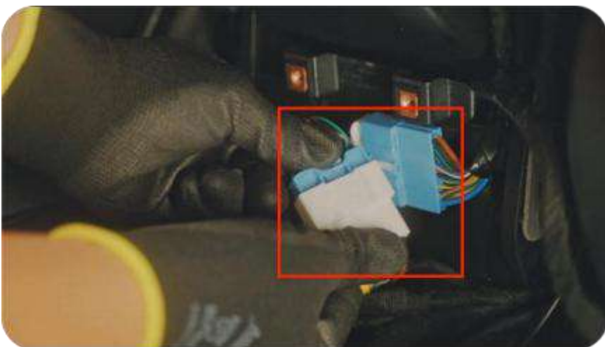
7. CANbus adapter plug and blue plug plug in together
