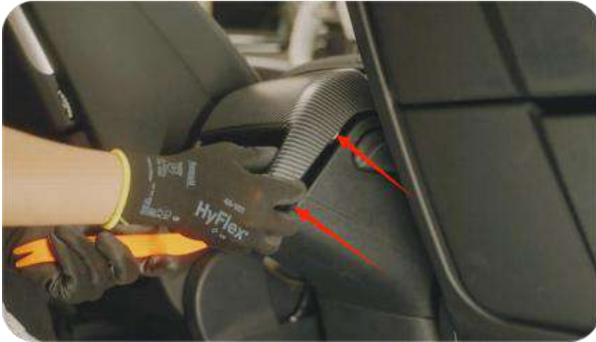
1. Remove the original rear air conditioning trim panel cover
