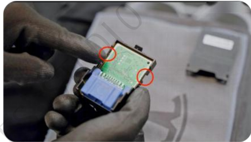
16. Remove these two clips on the electronic board.
