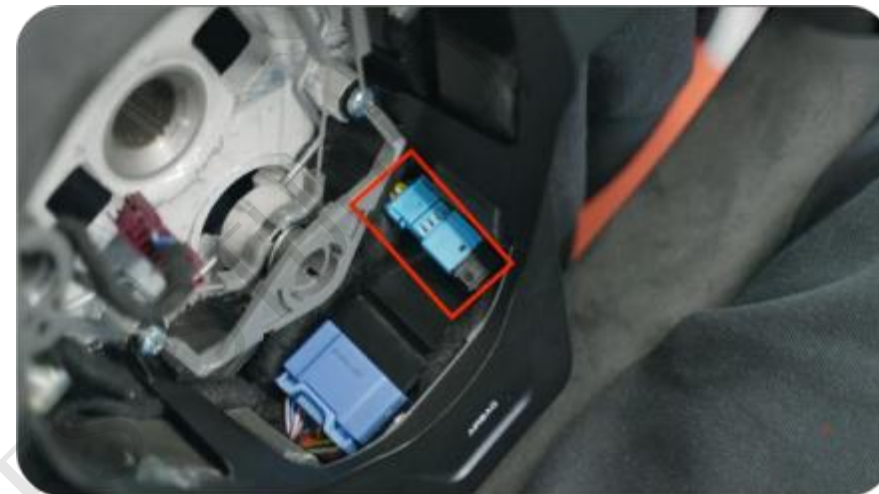
24. Plug in the heating connector and tuck it next to the control box
