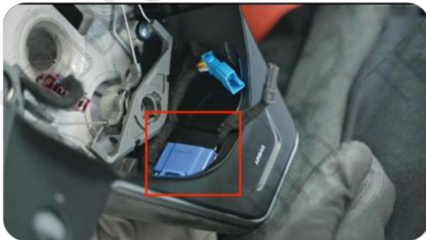
23. First, press the control box downwards at an angle and then press it upwards to secure it in place.
