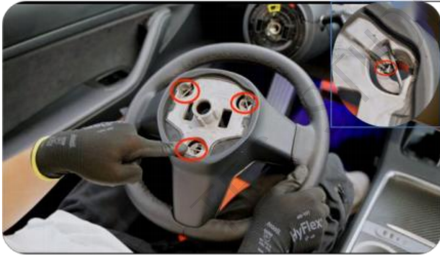
9. Use a Phillips screwdriver to remove the 6 retaining clips.
