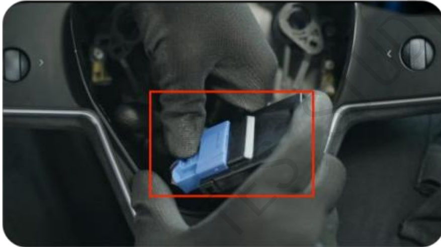
21. Insert the blue connector into the newly replaced control box.
