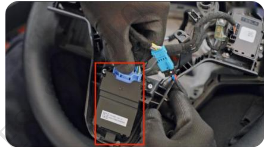
12. Disconnect the control box plug.
