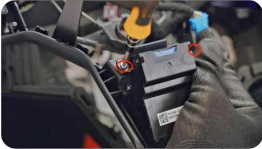
13. Use a T10 screwdriver to unscrew the 2 securing screws and then remove the control box.
