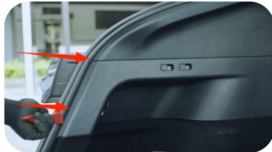
4. Use plastic trim removal take off the left trim of the trunk
