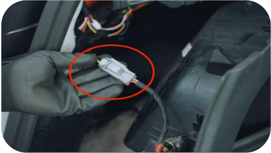
5. After remove the trim, find the plug of the original car cigarette lighter
