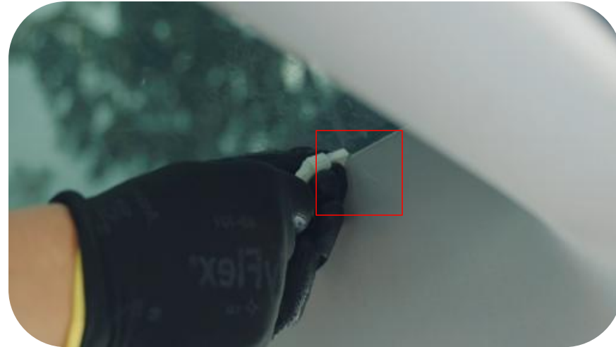
14. Connect the plug on the motor into the power plug that passes through the front (hide the plug in the roof).
