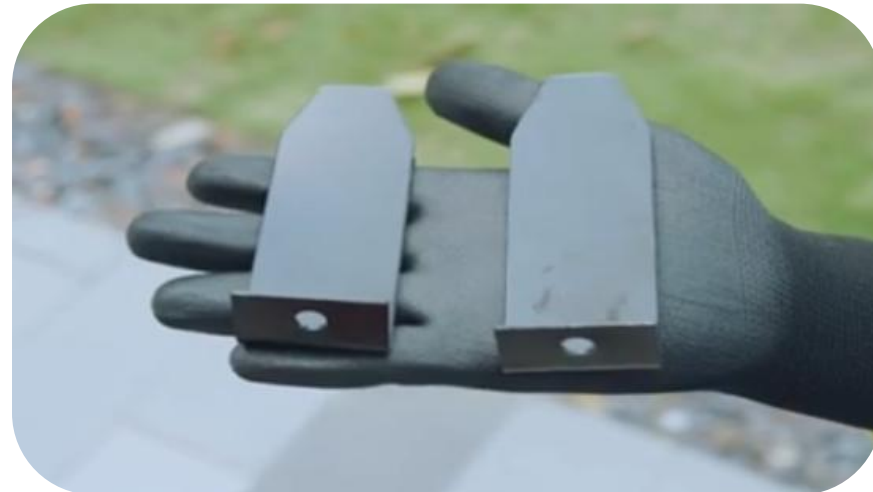
16. Insert these two latches into the gap between the glass and the trim above the front seat (left and right).
