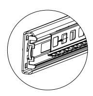
B: Insert the inside railway course on both sides of drawer on the outside railway course of cabinet at the same time. Two people must put the drawer flat and insert it slowly and synchronously. After inserting it to the end, pull it out slowly twice, the slide track works normally. If it works fails, please follow the slide track removal instructions, open it and reinstall it.
