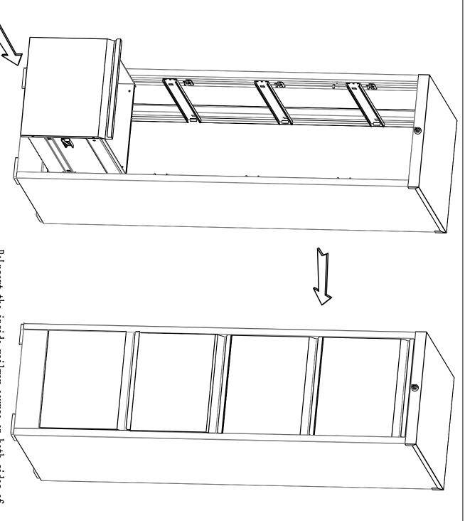
Must step: A First slide the steel ball to the front of cabinet's outer slide
