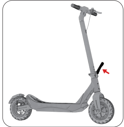
2. Close the folding handle in the direction indicated by the arrow.
