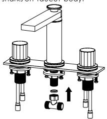
4. Attach one end of each of the shorter flexible hose to the adapter. Then attach the longer flexible hose to water supply. Turn on faucet for 1-minute to flush debris.
