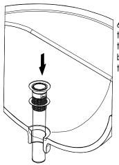
6.Insert the pop-up drain into the drain hole in the sink. Ensure the top gasket rests securely between the top of the sink and the top of the pop-up drain.
