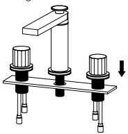
2.Re-install the rubber washer followed by the matal washer and lock-nut. Hand tighten then tighten further using a screw driverto tighten
