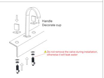
Remove the Decorate cup and put them on the basin holes. Connect the Control Water Bodies with Decorate cup from the underside of the basin holes, and tighten them. Finally install the Handles and tighten them. (Not to disassemble the valve by yourself, otherwise leakage will occur.
