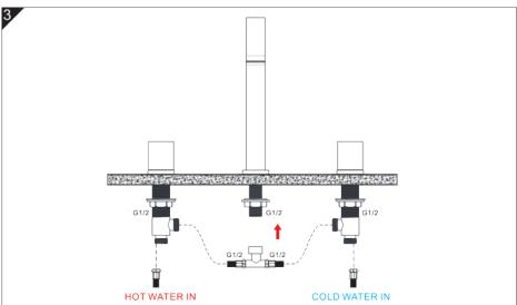
Connect one side of the Inlet Hoses to the Control Water Bodies, the other side to Tee, and tighten them. The red hose is for hot water and the blue hose is for cold water.
