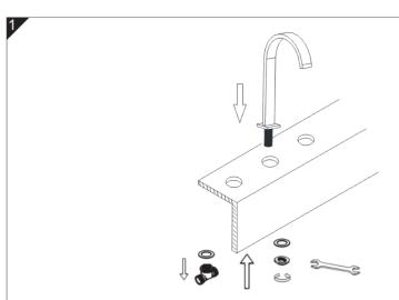
Put the Brass Part through the basin hole. Install Faucet Body Gasket and Mounting Nut in sequence and tighten the nut with a wrench. Then put Tee Gasket into Tee and connect Tee to Brass Part.
