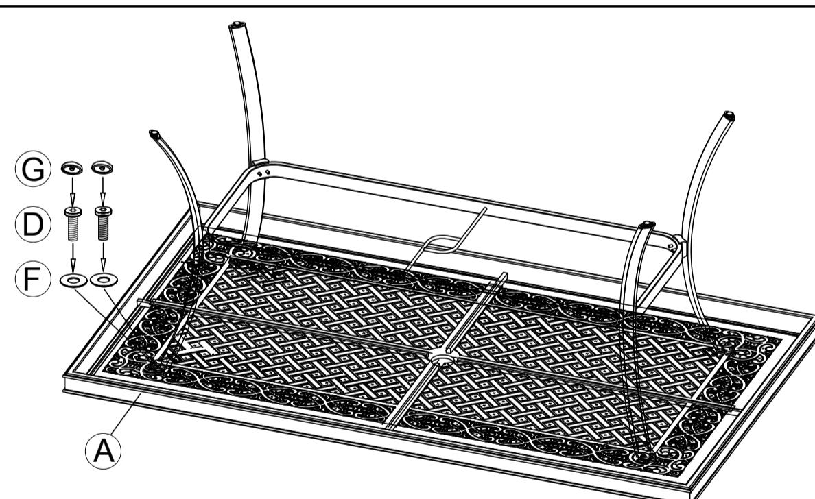
NOTE: Fix all the bolts in place, without tightening them first. After confirming the position of all the bolts, tighten the bolts and nuts. Each bolt must be tightened 3~4 revolutions only at a time and then move to another bolt until completely tightened, DO NOT TIGHTEN COMPLETELY one bolt first and then try to fix another bolt, as this operation will lead the other bolt hole to misalign.
