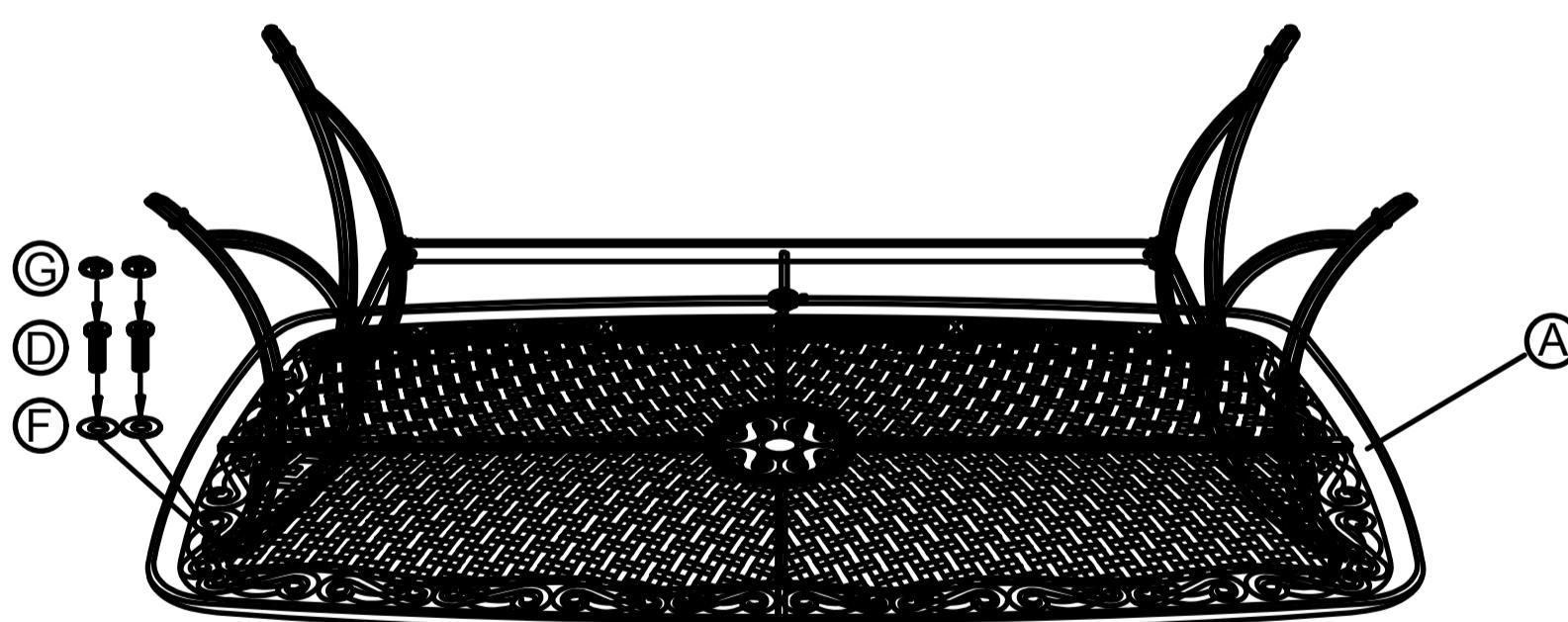
NOTE: Fix all the bolts in place, without tightening them first. After confirming the position of all the bolts, tighten the bolts and nuts. Each bolt must be tightened 3~4 revolutions only at a time and then move to another bolt until completely tighten, DO NOT TIGHTEN COMPLETELY one bolt first and then try to fix another bolt, as this operation will lead the other bolt hole to misalign.
