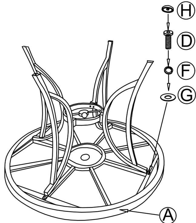
NOTE: Fix all the bolts in place, without tightening them first. After confirming the position of all the bolts, tighten the bolts and nuts. Each bolt must be tighten 3~4 revolutions only at a time and then move to another bolt until completely tighten, **DO NOT TIGHTEN COMPLETELY** one bolt first and then try to fix another bolt, as this operation will lead the other bolt hole to misalign.
