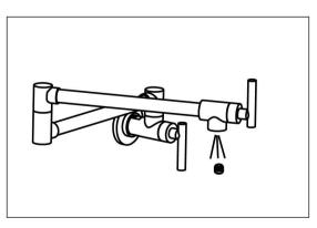
4. Remove the aerator, turn on the water and flush the faucet to check for leaks. If ok, then turn off the water and reinstall the aerator.
