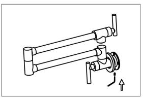
3. Fix the small set screw in the base and fasten the tap and the connecting pipe. Then adjust the cover to the base.
