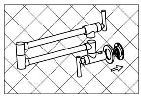
2. Hang the cover on the body, then install the faucet into the wall and tighten.
