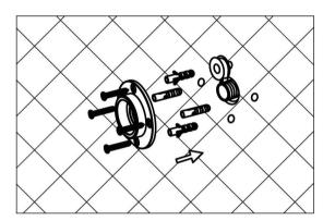
1. Wrap the thread on the pipe with the plumber's tape, then fix the pipe inside the wall. Fix the expansion screws into the wall and fasten the base onto the wall.
