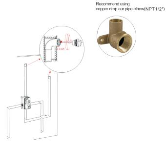
1:Recommend using Copper drop ear pipe elbow(NPT 1/2)
