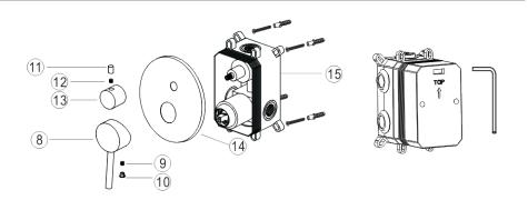
Please fix the ®Main body to the wall then remove the plastic protective cover and install ®Panel ® Water divider, ® Screw,® Water divider cup in the order. Finally you could install ® Handle, 9 Screw, ® Handle cup.
