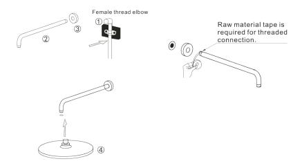
Connect top outlet ① to shower arm ②with proper fittings. To prevent damage, to finish on shower arm, insert wall end of shower arm into shower flange ③ before screwing arm into riser connection. Thread showerhead ④ onto shower arm. Apply tape to pipe threads on both ends. Do not overtighten showerhead. The showerhead is 360°swivel connection.
