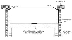
3. Place a thin layer of sealant on the supporting frame where it will contact the sink.
