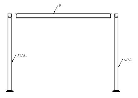
Step 2: Put A and A3 on both sides of B first, then repeat the same steps for A1 and A2, installation instructions in step 3
